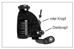
You switch on the tire dynamo by pressing the red button. To switch off the dynamo move it away from the wheel.
