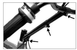
On the stem you will find 3 clamping screws for adjustment.
