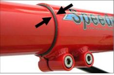
The plastic spacer between front boom and main frame must be visible at all time.
