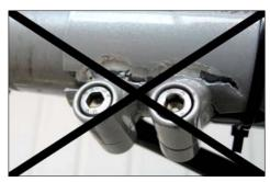
If the spacer is missing or not alligned properly or the screws are tightened too much, the frame can break!
