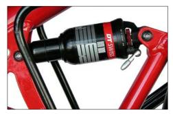
Air Shock DT-Swiss XM180 Damping ist adjusted with the red knob at the rear end. The shock must be installed with the lock-out lever facing down to avoid a collision of lever and frame when the suspension is moving.
