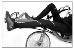
Adjust the front boon so that your knee will not be fully straightened when pedaling.
