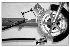
Check that thre is at least a 5 cm (2")clearance between the end of the chain tube and other parts of the drive train.
