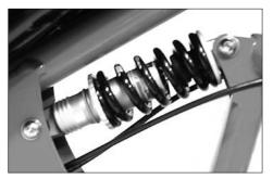
Suspension element DV-22 with fixed damping rate.
